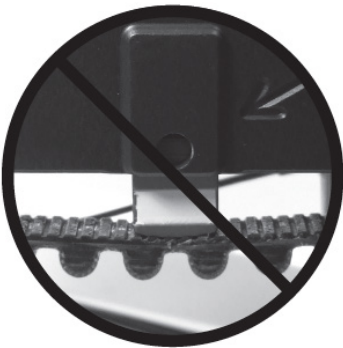
Illustration 1: Incorrect belt tension
