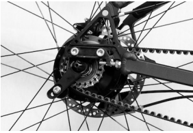
Illustration 3: Side view of the installed Snubber
