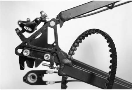
Illustration 1: Opening the frame to mount the belt
