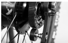
Illustration 1: Rohloff SPEEDHUB 500/14 with Snubber
