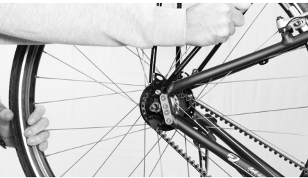
Illustration 3: Correct alignment of the belt
