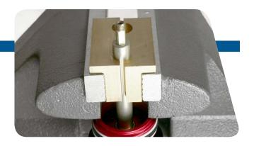
Monarch™ RT3: Install the main piston assembly that was removed in step 5 onto the damper shaft. Use your fingers to squeeze the shims and center the shim stack under the main piston. Use a small pick to center the shim stack along the inside edge of the main piston.
