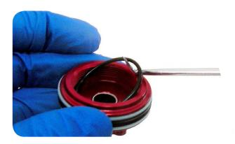
Use a 1.5 mm hex wrench to push the compression ball out of the backside of the seal head through the bleed port.
