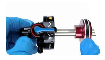
Use a vise block with the 10 mm shaft clamp to clamp the shaft into a vise.
