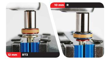
Use a small wrench or pick to slide the main piston assembly off the shaft and onto the tool.
