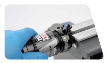
Remove the shock from the vise. Turn it over and clamp the damper body eyelet in the vise.
