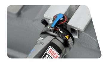
If the shock is collapsed so that a minimal amount of damper body is visible, there is still air pressure in the air can.
