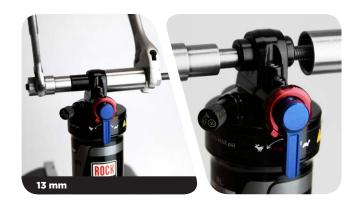
Unthread the catcher from the threaded rod and remove the tool from the shaft eyelet.
