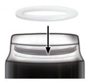
7 Orient the new dust wiper seal step side up. Install it into the dust wiper seal groove at the top of the air can.
