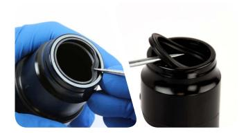
Use a pick to remove the two backup rings from the second deepest groove inside the air can.
