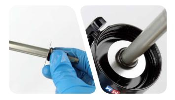
17 Use your fingers to remove and replace the o-ring located inside the shaft eyelet threads.
