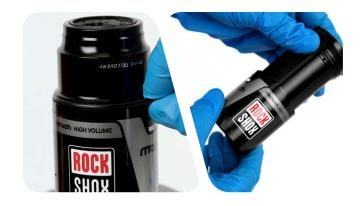
High Volume Air Can: Use your fingers to remove and replace the high volume sleeve o-rings.
