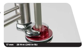
Allow air bubbles to escape from the bleed port in the seal head.
