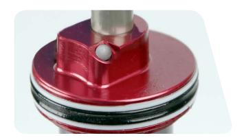
Use a 2 mm hex wrench to thread the bleed screw into the bleed port until you feel it touch the compression ball, then tighten the bleed screw an additional ½ turn.
