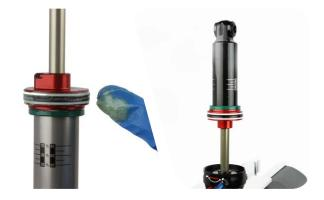
2 Inject 0.5 mL of Maxima® Maxum4 Extra 15w 50 into the air can before installing the air can onto the damper. Firmly press the air can down until the sealhead/air piston is inserted into the air can.
