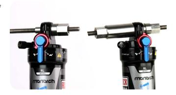
2 Clamp the catcher in a vise or hold it secure with a 13 mm wrench.
