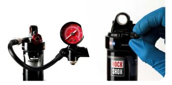
DebonAir™ Air Can only: Use a shock pump to pressurize the shock to the desired air pressure. After adding air to the shock, the pressure will need to be equalized between the shock chambers.
