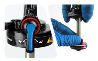
Use your hand to install the seal head/air piston onto the damper body.
