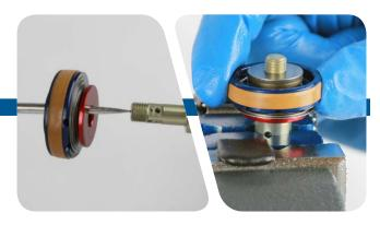
17 Apply a thin layer of Loctite® Threadlocker Blue 242® only on the threads of the nut, then thread the nut onto the damper shaft.
