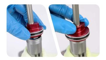
Use a torque wrench with 17 mm crowfoot to tighten the seal head/air piston to 28 N·m (248 in-lb).
