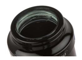
**9 High Volume Air Can:** Remove the retention o-ring from the high volume sleeve. Firmly grip the high volume sleeve and slide it off of the air can.
