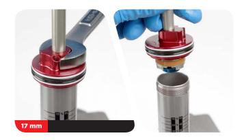
**Z** Remove the damper body from the vise and pour the fluid into an oil pan.
