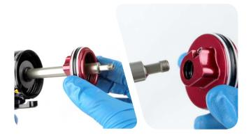
Use a pick to remove and replace the internal seal o-ring located in the internal seal gland.
