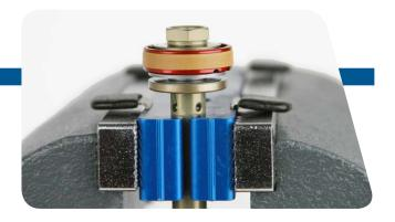
**4** Monarch<sup>™</sup> RT3: Use a 12 mm socket wrench to remove the piston nut.
