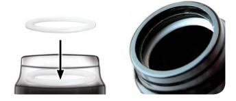
Apply a small amount of RockShox Dynamic Seal Grease to the new quad seal and install it above the backup ring in the second deepest groove.
