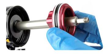
Use a vise block with the 10 mm shaft clamp to clamp the shaft into a vise.
